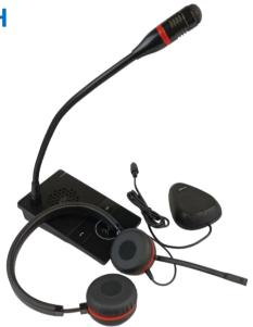
The OP-6505H is a speech transfer system designed to improve communication at fixed screen counters. Integrating a DSP technology a Full duplex system and a headset with microphone, it is particularly efficient when communications are altered by the presence of double glazing, security screen, or other counter security systems.
